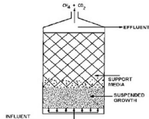
Figure 1. Anaerobic Filter
