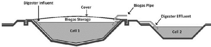
Figure 2. Covered Anaerobic Lagoon
