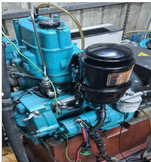
Figure 1. Experimental setup of the diesel engine used for performance testing
